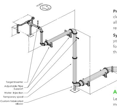
**Pneumatic high-quality target inserters.** Test steam-blow cleanliness reliably and efficiently. Testing can be done on all pipe diameters. Our system simplifies target insertion and removal, and eliminates sticking risk.
