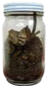
Debris removed during Hydro Pig cleaning of a lube oil system
