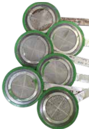
Screens pulled during a conventional oil flush
